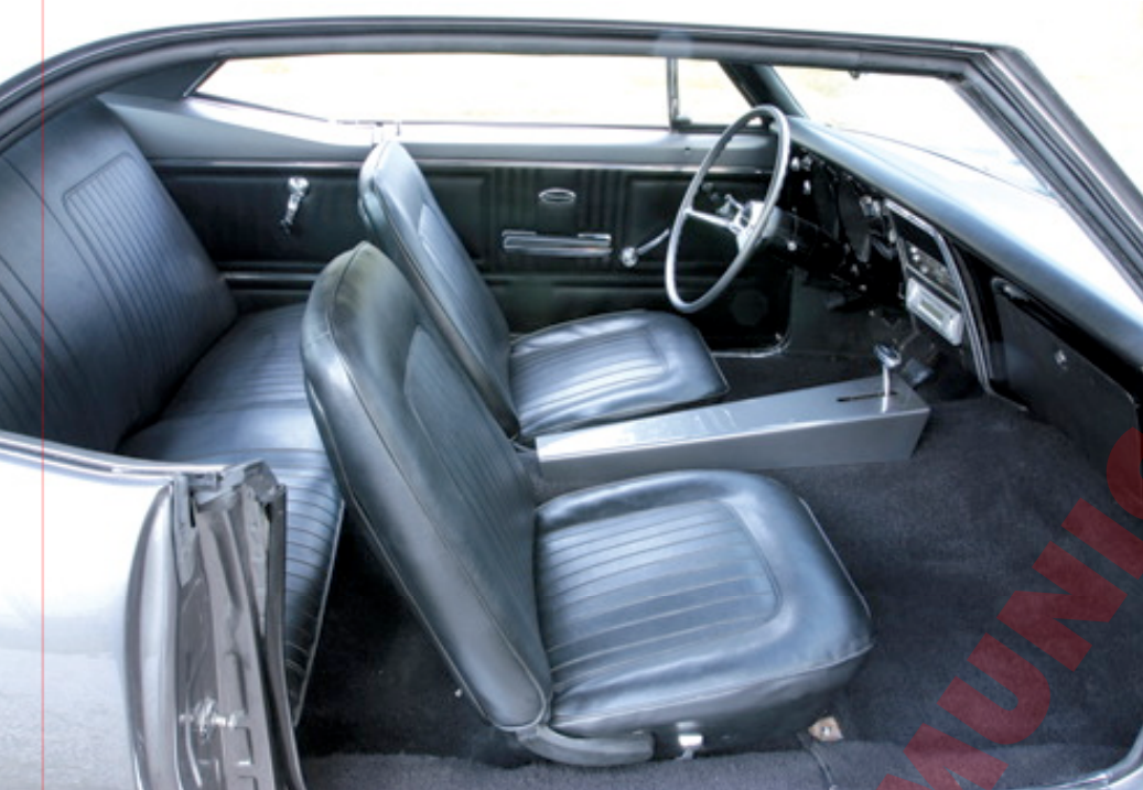
Bob Allfrey wrapped the original bucket seats with new black vinyl and also re-covered the door panels. The console between the seats was handmade by Derick Samson and painted Iron Gray to match the exterior. A '57 Chevy steering wheel replaces the stocker and has a custom horn button that features a "Stealthed" emblem. The dash and gauges are in their original configuration, and a Sony CD player is in place.
